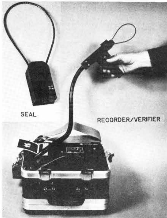
FIBER OPTIC SEAL (upper left) is checked for tampering by attaching it to the verifier head (pistol-shaped device containing light source and optics), which is connected to the recorder/verifier. The recorder/verifier, mounted in a case, contains film, optics, camera, and controls. The verifier head, triggered automatically by insertion of the seal, shines light onto the ends of the seal's cable, and a Polaroid photo of the light dot patterns is produced. The patterns are then compared to the seal's original signature.
